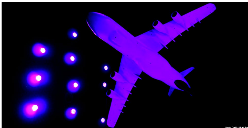
ISSI LEDs Mounted in AEDC 16T Wind Tunnel During Pressure Sensitive Paint Tests, Photo Credit US Air Force
