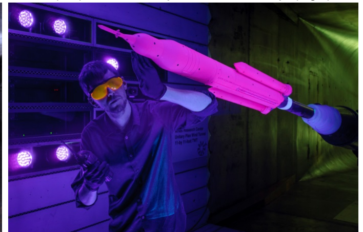
Preparation of SLS Rocket Model (Left), SLS Rocket Model Glowing Pink Under UV LEDs (Credit: D. Hart / NASA Ames Research Center)
