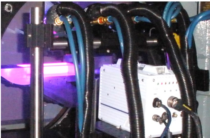
ISSI LEDs Mounted in Cavity Acoustics Fast PSP Test (Left), Courtesy US Air Force Research Laboratory, ISSI Water-Cooled LEDs mounted in the ARA Transonic Wind Tunnel (Right), Courtesy of ARA, Bedford, UK
